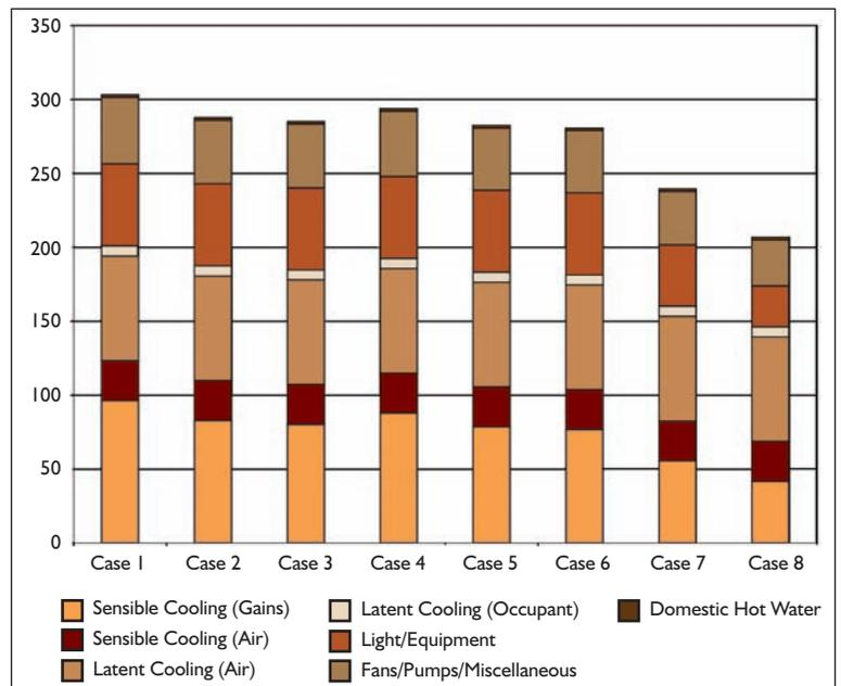
Figure 1: Total building cooling and thermal loads by end use (kWh/m<sup>2</sup>·yr).
