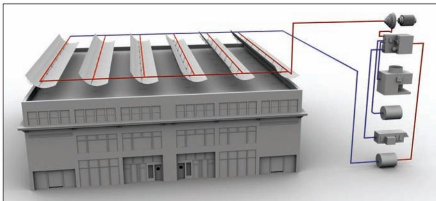
Figure 5: Parabolic trough solar collection system with steam turbine generator, absorption chiller and domestic hot-water heating.
