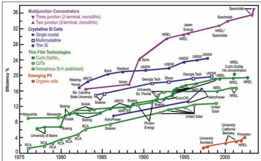
Figure 4: Photovoltaic cell conversion efficiencies improvement from 1975 through 2003.<sup>4</sup>
